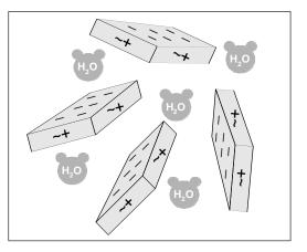
For most smectites, the speed with which platelet separation occurs is directly related to the amount of energy introduced during hydration. Both mechanical and thermal energy will accelerate hydration: high shear mixing or the use of warm water will reduce hydration time. The presence of dissolved substances in the water will prolong hydration time by inhibiting the osmotic swelling essential to platelet separation.
